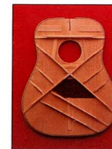
Symmetrical X bracing pattern for "dreadnought" style guitars.
